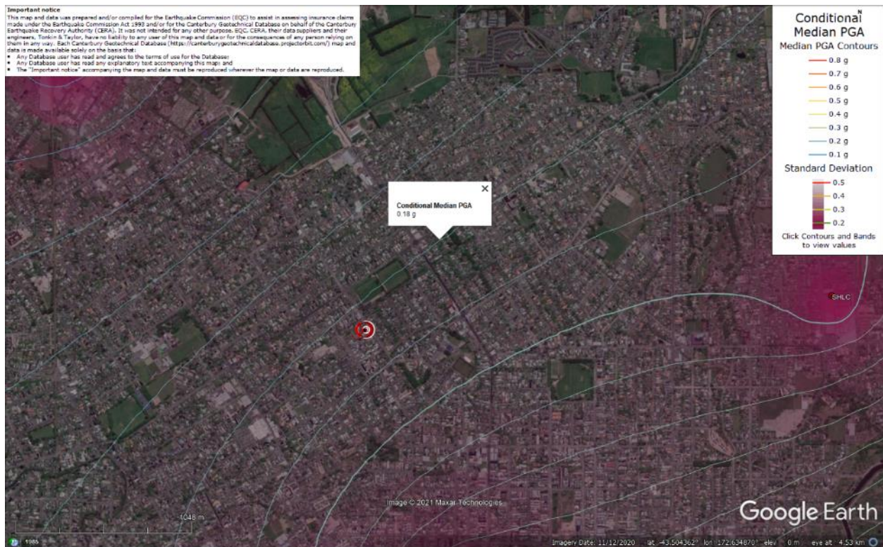
Figure 42: PGA for Jun-11 EQ (st. dev. = 0.350-0.375 ln units).
